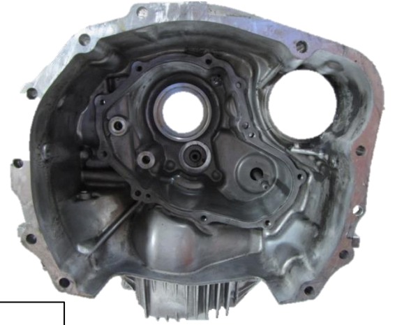
Stator Support Removed
